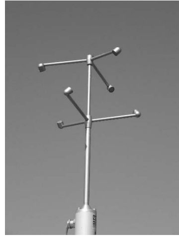
Fig. 6.14. Sonic anemometer USA-1 with inclined paths and omni-directional construction (Photograph: Foken)
