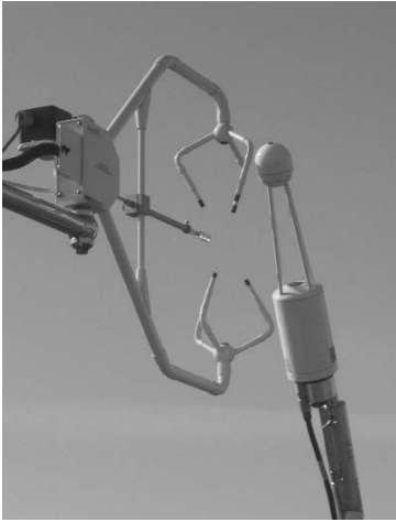
Fig. 6.13. Sonic anemometer CSAT3 with inclined measuring paths and large inflow sector; additionally an IR gas analyzer LI7500 and a sensitive temperature sensor are mounted (Photograph: Foken)
